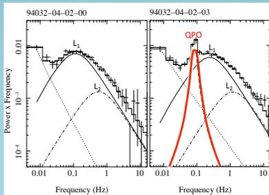
Fig. 2. Example of low-luminosity ( $L_x = 2.31 \times 10^{36}$  erg  $\text{s}^{-1}$ , left panel) and high-luminosity PSD ( $L_x = 2.50 \times 10^{37}$  erg  $\text{s}^{-1}$ , right panel) with fitted components: a power law (dotted line),  $L_1$  (solid line),  $L_2$  (dash-dotted line) and the QPO (red solid line). On the top of each panel the RXTE observation ID is reported.
